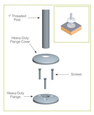
For Millwork Counter MW2: Narrow Flange
